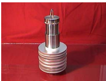
Figure 1. A typical corrosion test rack with coupons.
